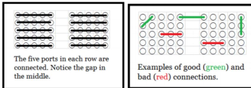
Figure 5 Examples of good and bad connections on a breadboard. Image courtesy of 2013 SPS SOCK.
