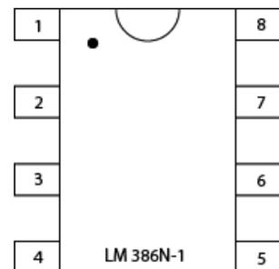
Figure 4 physical pin out of amplifier.
