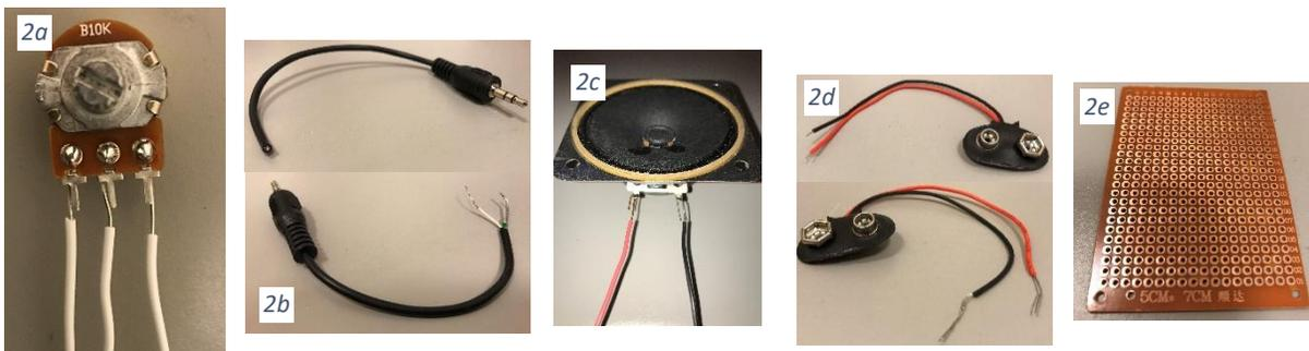
Figure 2 **a)** The potentiometer wires soldered on **b)** the headphone jack wires before and after wire stripping and soldering **c)** wire speakers soldered **d)** 9V battery connector before and after wire stripping and soldering **e)** a basic protoboard which can be used to solder the circuit together for a more permanent circuit.
