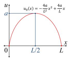
Figure 1: Initial heat distribution along the rod.
