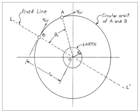
Figure 1. Spacecraft B is beginning its transfer to a full elliptical orbit around planet Earth.
