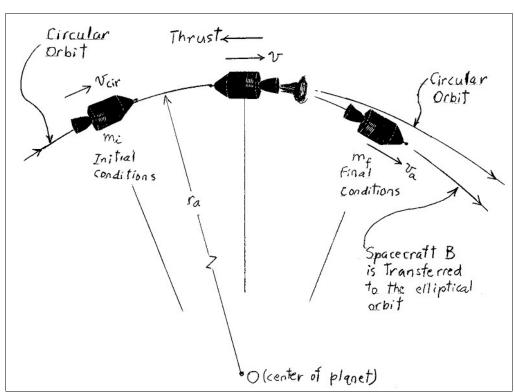
Figure 4. Spacecraft B is reducing its speed by firing the rocket in reverse position. The firing occurs between the initial and final conditions shown.
