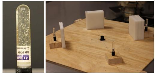
FIGURE 2. Left: An exposed bubble detector used for counting. Right: Experimental setup.
