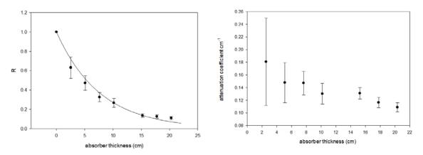
**FIGURE 3.** Left: Transmitted over incident flux vs. absorber thickness. Right: Absorption coefficient  $\mu$  vs. absorber thickness.
