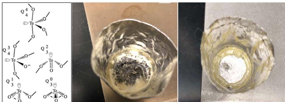
**FIG. 1.** Left:  $Q_m^n$ , where  $m = 3,4$  identifies the total number of oxygen bonded to the tellurium atom and  $n = 0-4$  is the number of bridging oxygen bonded to the tellurium atom.<sup>11</sup> Right: Tellurium dioxide crystal (left). Pure tellurium dioxide glass made with IQ technique (right).
