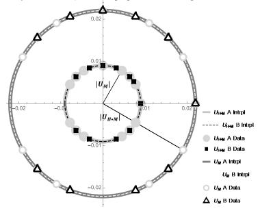
**FIGURE 2.** Magnetostatic energy in a.u. of single Mn atom cubic system as a function of  $\vec{M}$  orientation. Distance from the origin to the point is  $|U_M|$  or  $|U_{H \cdot M}|$  (see legend). Legend entries denoted "A" signify  $\vec{M}$  orientation in the x-y plane ( $M_z = 0$ ); those denoted "B" are beholden to the plane generated by vectors {0,0,1} and {1,1,1}. "Intrpl" = interpolated function of circle.
