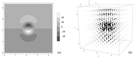
**FIGURE 1.** (a) Magnetic charge density  $\rho_M$  in a.u. of Mn 3*d* orbital resultant of magnetization pointing in z-direction (x-z plane,  $y = \frac{a}{2} a_0$ ). (b) Vector field of magnetization  $\vec{M}$  (gray) and magnetic field strength  $\vec{H}$  (black) of Mn 3*d* orbital. Values in a.u.
