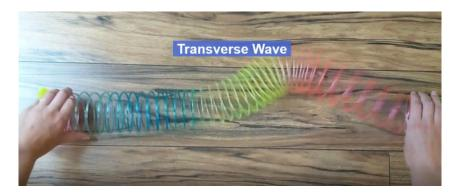
Figure 3a. Image of slinky demonstrating a transverse wave
