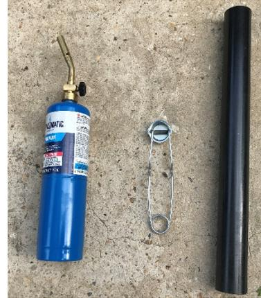
*A great example of resonance, heating up metal mesh placed in a pipe will cause the pipe will sing at a predictable frequency.*
