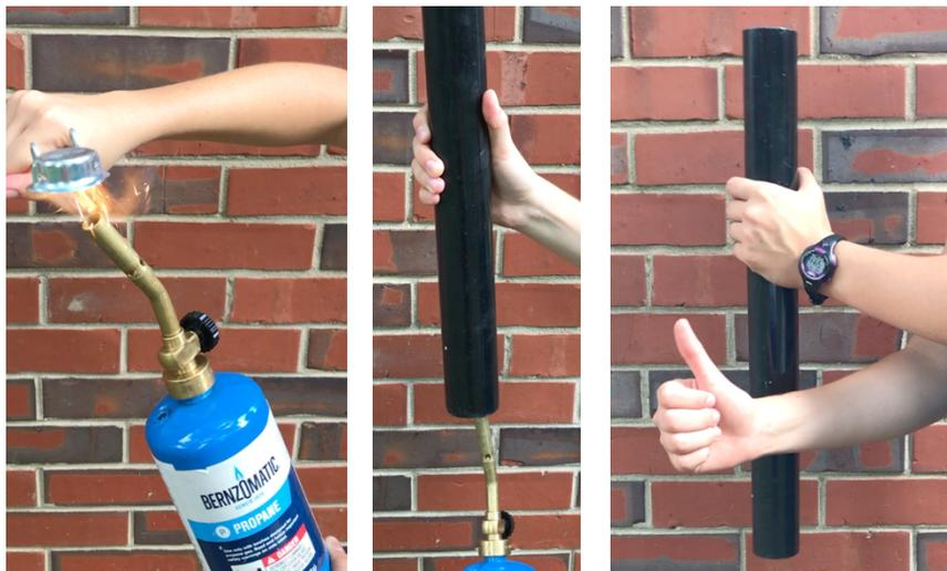
Figure 2 Light the propane, heat up the mesh in the tube, and hear it sing (as long as the pipe is vertical).
