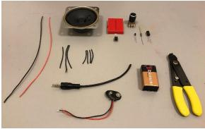
Figure 1 Materials provided needed to create an audio amplifier
