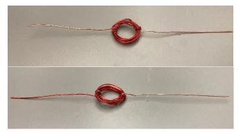
Figure 3 The copper is exposed on 3 out of 4 sides of the coil ends.
