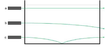
stirring; since the corn syrup was placed evenly at the bottom of the tank then the water was slowly added on top, the solution should have a greater concentration of syrup at the bottom of the tank. Thus, there should be a gradient in the index of refraction with depth.
