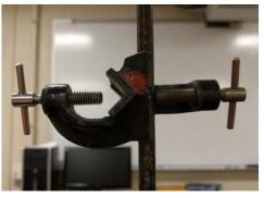
Figure 2: Double-ended bosshead clamp
