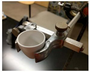
Figure 4: Mounted ceramic crucible.
