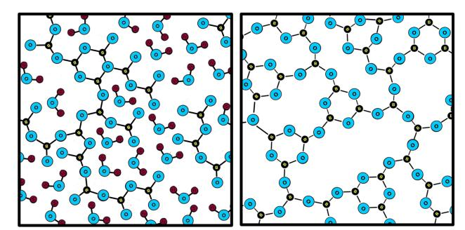
Figure 12: All hydrogen will bond in pairs to free oxygens, creating water molecules, while the trigonal borate and boroxol rings bond to one another forming the final glass network.
