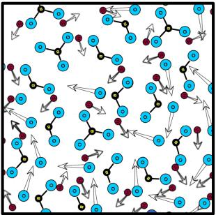
Figure 11: With the addition of heat, bonds between the hydrogen and some oxygen break, forcing the hydrogen and oxygen to move around. Boroxol rings and trigonal borate are freed move around.
