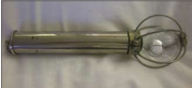
Figure 4. Mercury lamp used by Ralph Alpher while testing torpedoes in Puget Sound during World War II. If it was necessary for the testing crew to abandon their wooden boat, this lamp would emit a faint blue signal at night that could be seen by rescue teams.
