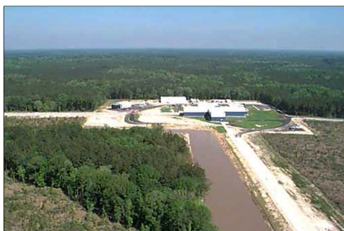
LIGO in Livingston, LA, one of two sites for this gigantic gravitational antenna. There are two, perpendicular 4-kilometer arms in this interferometer, one stretching toward the reader in the photo, while the other continues beyond the image edge to the left.
