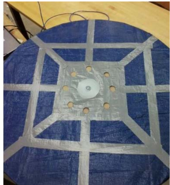
Figure 2: The bottom of the hovercraft. The holes in the middle are where the air escapes to inflate the skirt and the duct tape dampens the vibrations of the skirt.
