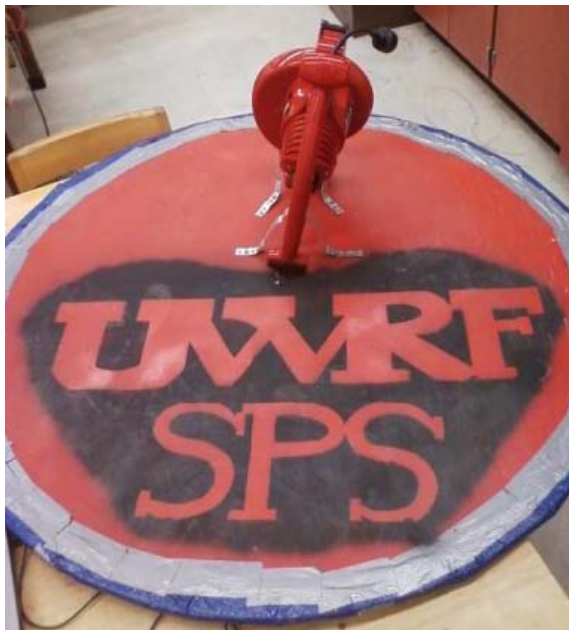
Figure 1: The top of the hovercraft. The leaf blower is directed into a hole in the platform in order to inflate the skirt
