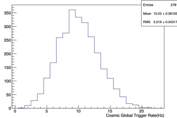
**FIGURE 8.** Global cosmic trigger rate had been continually measured by a VME scaler module from CAEN. The global coincidence trigger rate, of six top and six bottom scintillators, found to be  $(10.05 \pm 3.124)$  Hz matching the simulation value that is of 10.45 Hz. The distance between top and bottom scintillators is 19.2 cm.
