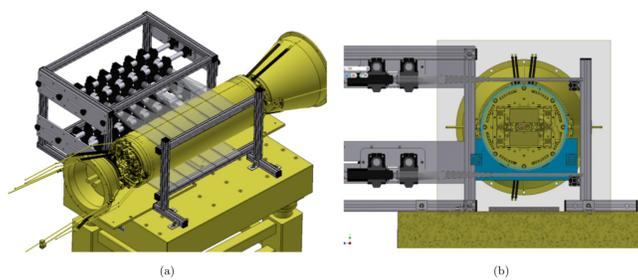
**FIGURE 2.** Front view (a) and a side view (b) of the cosmic trigger system frame, with its 12 scintillators. The pictures also show the way at which the VXD is fixed on the commissioning granite table at KEK.
