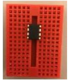
Figure 3 Inserting the LM386 to the breadboard. You want the op amp to be straddled in the middle so each pin is on a separate row.
