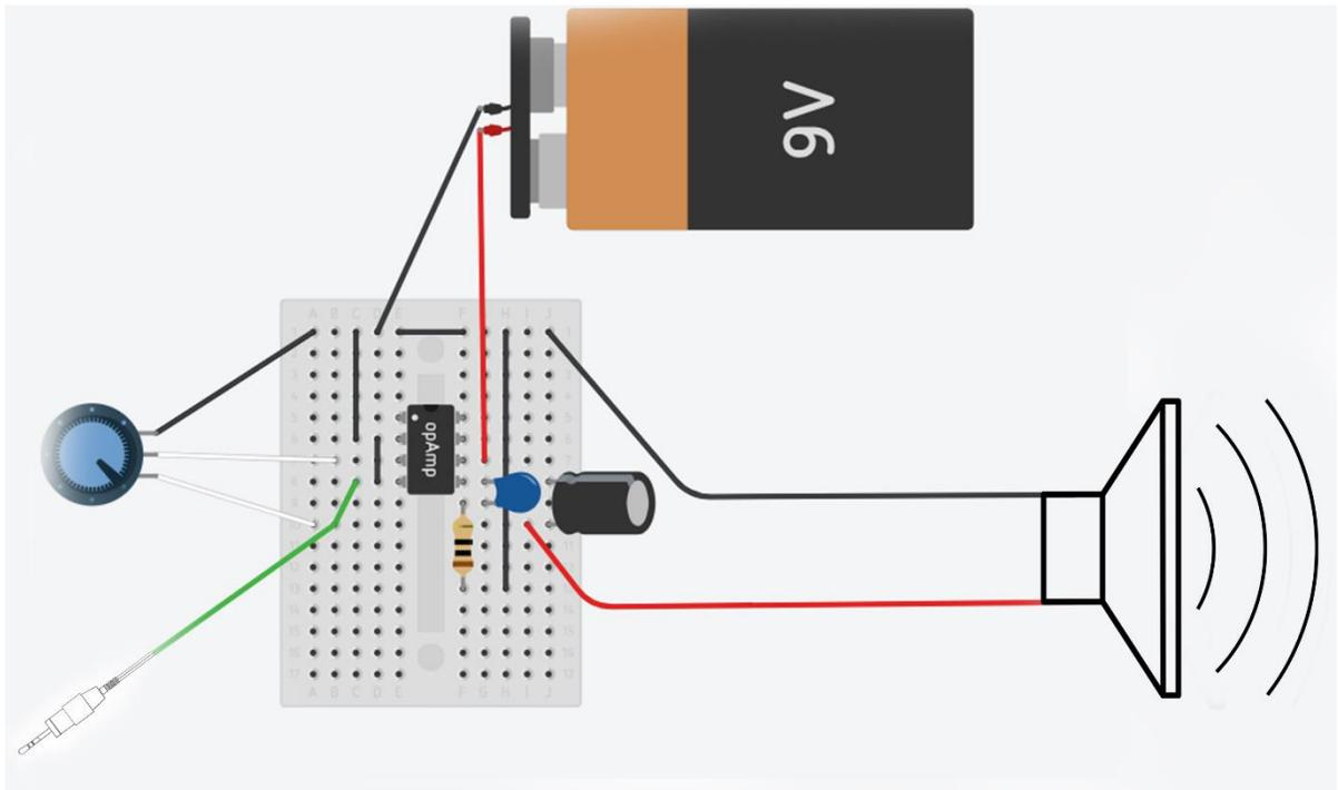
Figure 4 A physical visualization of the circuit. All the black wires indicate they are for grounding, the green wire is the different wires in the speaker. The blue capacitor is the  $0.1\ \mu\text{F}$  capacitor, while the big capacitor is the polarized  $220\ \mu\text{F}$  capacitor. The longer end of the capacitor should be pinned on the row attached to the op amp.
