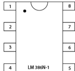
Figure 4 physical pin out of amplifier.
